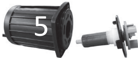
Remove rotor from pump house
