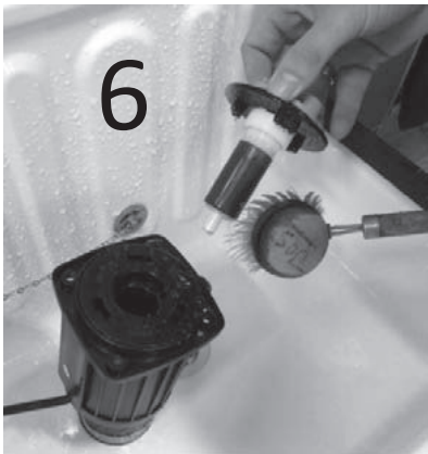
Clean rotor with water and brush
