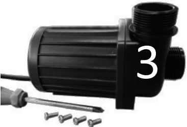
Remove the screws from pump house
